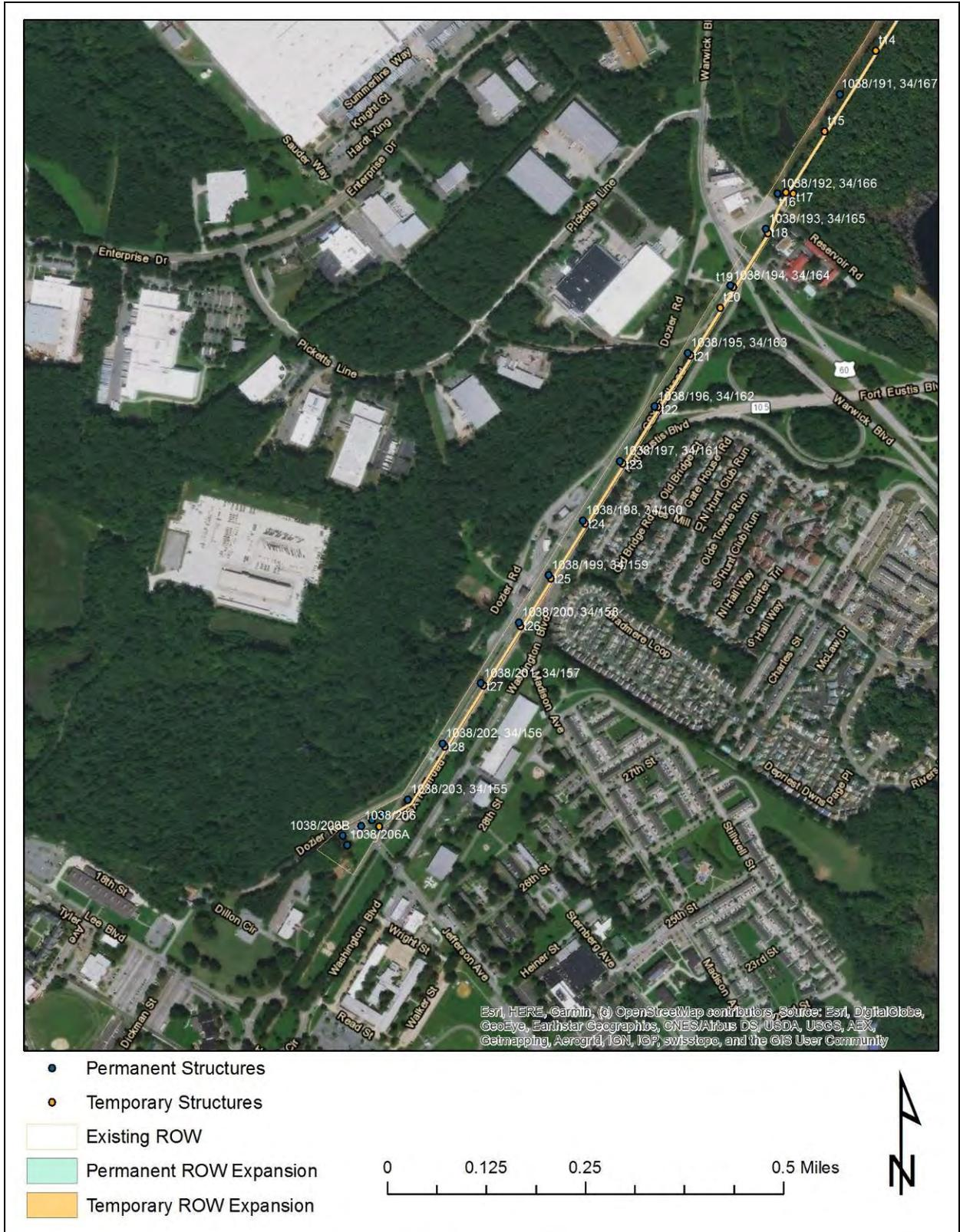
Figure 1-4: Detail of proposed permanent and temporary structure locations with ROW expansion (south half of alignment). Source: Dominion
