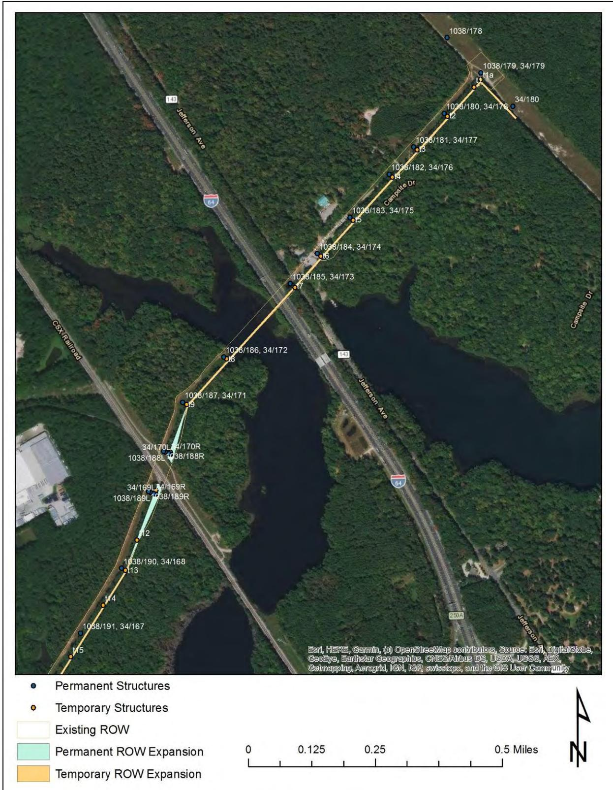
**Figure 1-3: Detail of proposed permanent and temporary structure locations with ROW expansion (north half of alignment). Source: Dominion**
